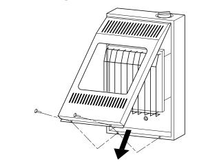
Figure 8 - Removing Front Panel Of Heater
